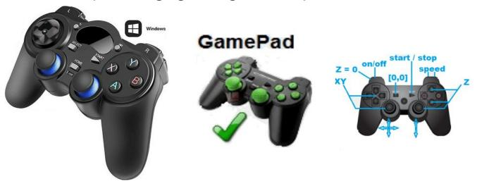
Left stick is used to control the XY axes,
