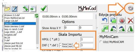
Loading a drawing into the import window is done by clicking the buttonbeforehand to indicate which layer colour is the 'active' one.
