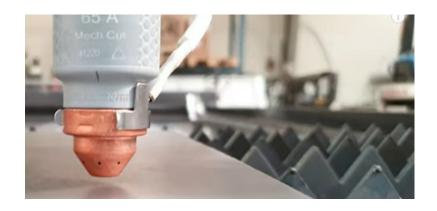
Position the torch at the material breakthrough height (or at the cutting height for Automatic THC mode), switch on the plasma with the SPACE KEY and start the feed with one of the arrows (screen or keyboard) of the X/Y manual operation (Up / Down / Left / Right).
