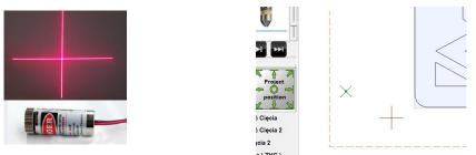
If a laser pointer / crosshairis mounted on the machine and its offset is specified, the material positioning options (Material Position) are performed relative to it and not to the plasma torch.
