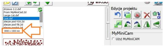
If the size does not agree here (it usually deviates significantly from the expected size by incorrectly interpreted units), force the use of metric or imperial units in the import options, or change/adjust the import scale (default is 1):
